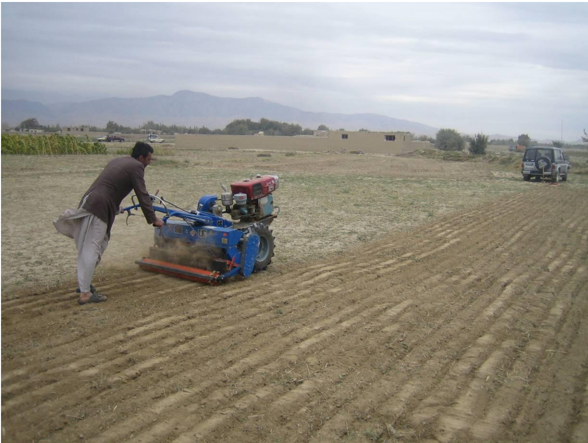
On-farm strip tillage demonstration using C2WT cultivating seed drill in irrigated wheat, Balkh province.
