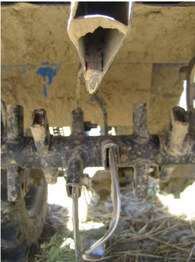
Blades are only where seed will drop from opener.
