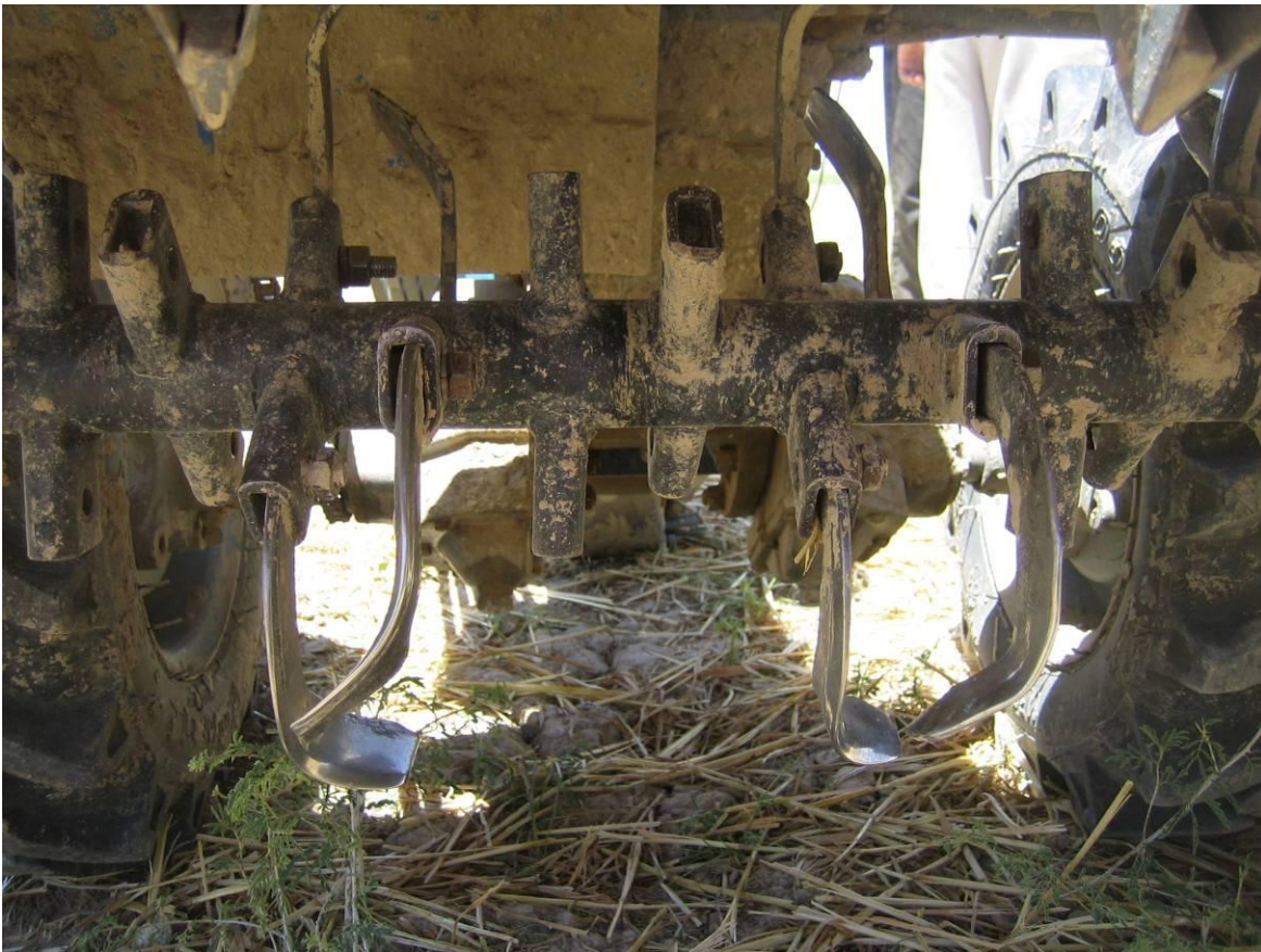
Blade setup on C2WT cultivating seed drill for strip-tillage.
