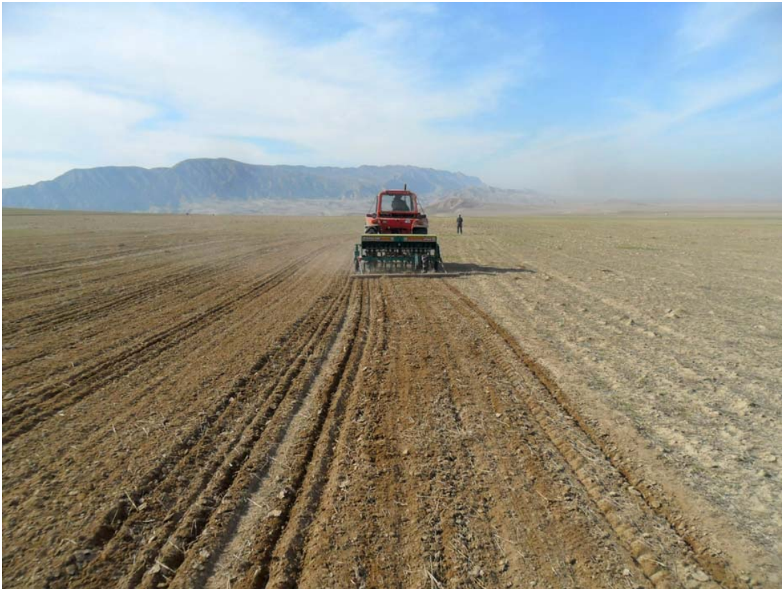
Photo 7 4WT seeder on rainfed land in Jawzjan, 2013
